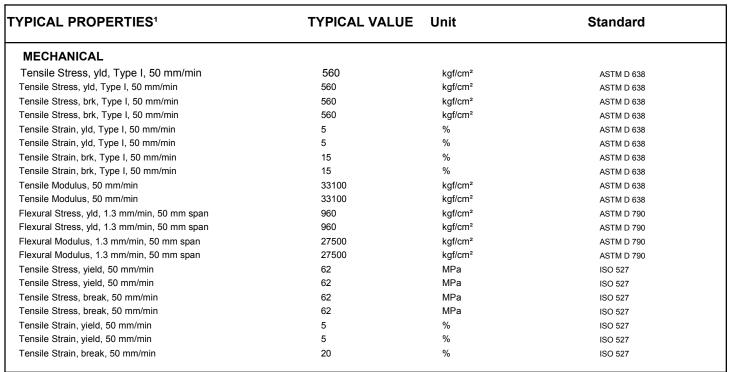
(1) Typical values only. Variations within normal tolerances are possible for various colors. All values are measured after at least 48 hours storage at 23°C/50% relative humidity. All properties, except the melt volume and melt flow rates, are measured on injection molded samples. All samples tested under ISO test standards are prepared according to ISO 294.
